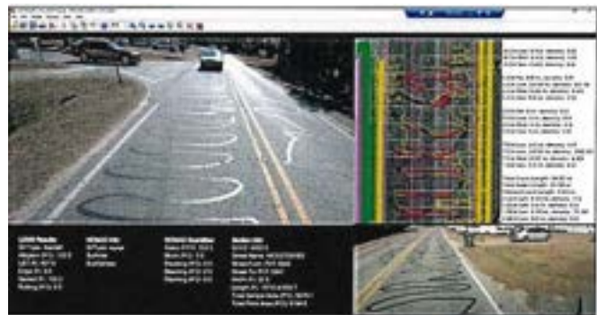
New QA Tool! IMS QC/QA interface for manually reviewing automated distress detection and classification results.
