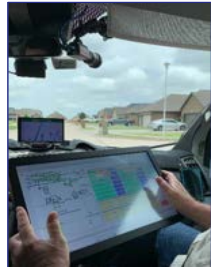
IMS' customizable touchscreen NOMAD™ interface for entering notes and supplemental field data.
