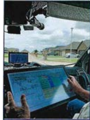
IMS' customizable touchscreen NOMAD™ interface for entering notes and supplemental field data.
